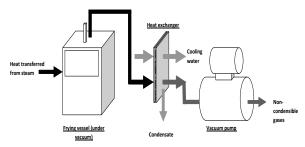
Figure 1. Schematic diagram of the vacuum frying system.
